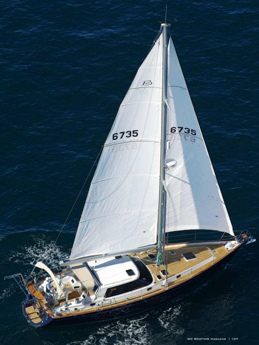
cruiser – it is so easy to sail. Unlike many other imported yachts, the Buizen is not a cruiser/racer – it is a genuine cruiser with a 16 tonne displacement, of which 5.5 tonnes is ballast in the flattened lead bulb. The yacht has a fin keel of 3.5 metres in length.
